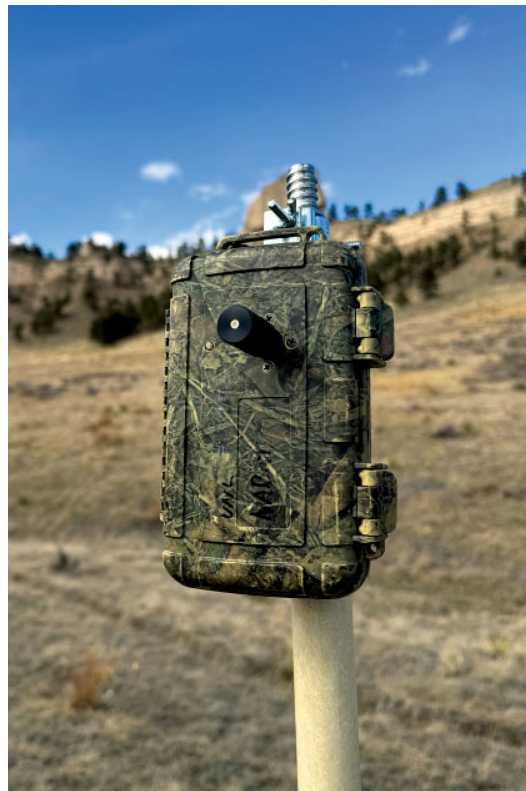
A Titley AnaBat Express stationary acoustic monitor deployed at Fort Robinson State Park. PHOTO BY DEREK KRUEGER
