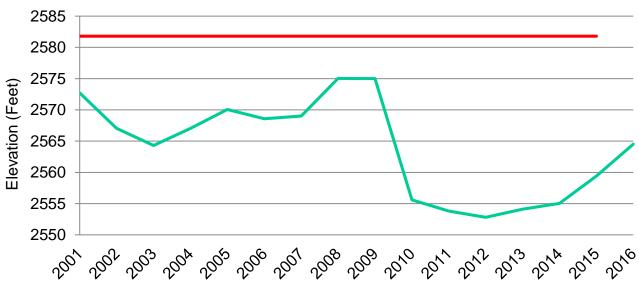
Water levels have been extremely low at Red Willow due to structural repairs of the dam that began in 2009. Construction was finished in 2013 and lake elevations have started the road to recovery. The green line indicates annual mean elevation and the red line indicates the top of the conservation pool elevation. Current elevation data can be found by following this hyperlink: <u>Current Elevation</u>
