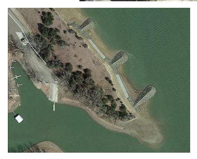
Left: An aerial photo of the trail 1 boat ramp area. Three perpendicular breakwaters will protect the mouth of the bay and prevent further sedimentation due to wave action.
