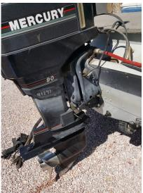
Don't forget to lower your outboard motor to drain all the water from your lower unit before leaving a boat launch facility.
